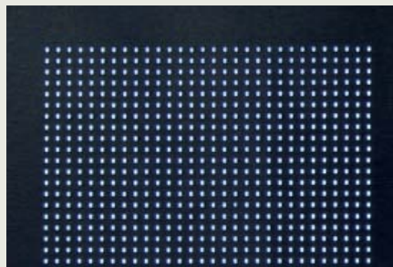
Drilling microstrainer pattern in 0.3 mm stainless steel
