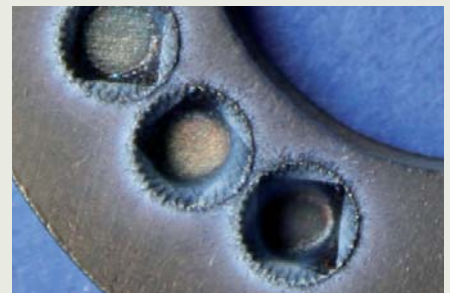
Deep engraving in a refractory Titanium alloy
