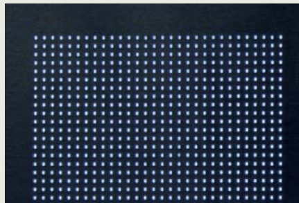
Drilling microstrainer pattern in 0.3 mm stainless steel
