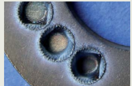
Deep engraving in a refractory Titanium alloy ablation rate 3.5 mm 3 /s
